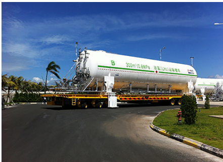
Liquid Hydrogen Storage Tanks
